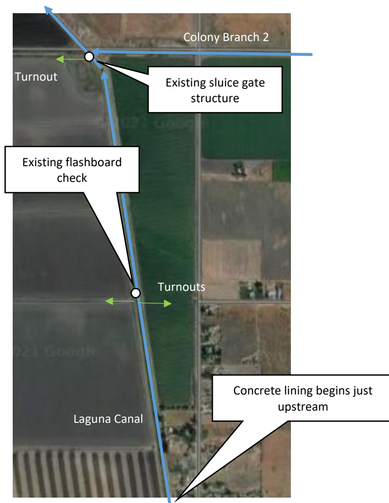
Figure 27. Existing conditions along the Laguna Canal just upstream of the convergence with Colony Branch 2
