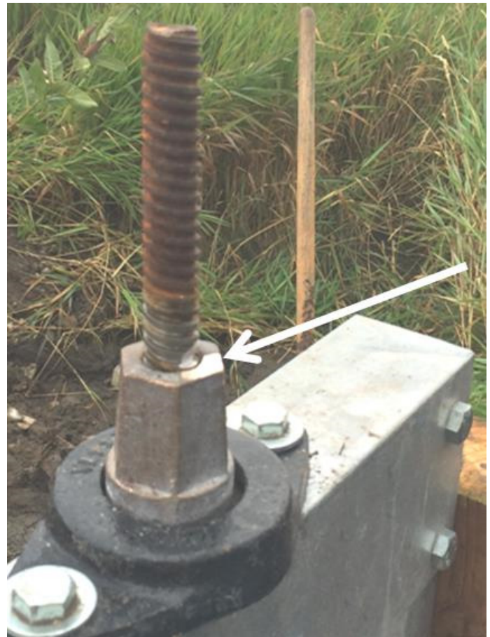
Figure 6. Proper cut in shaft to mark the “zero” opening
