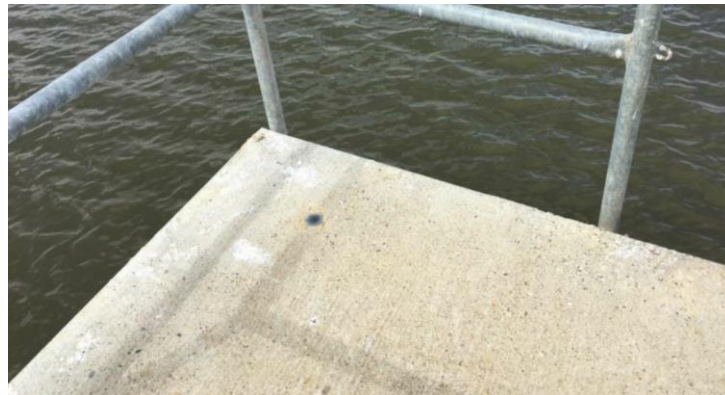
Figure 5. Monument found adjacent to the reservoir outlet gate; assigned an elevation of 100'
