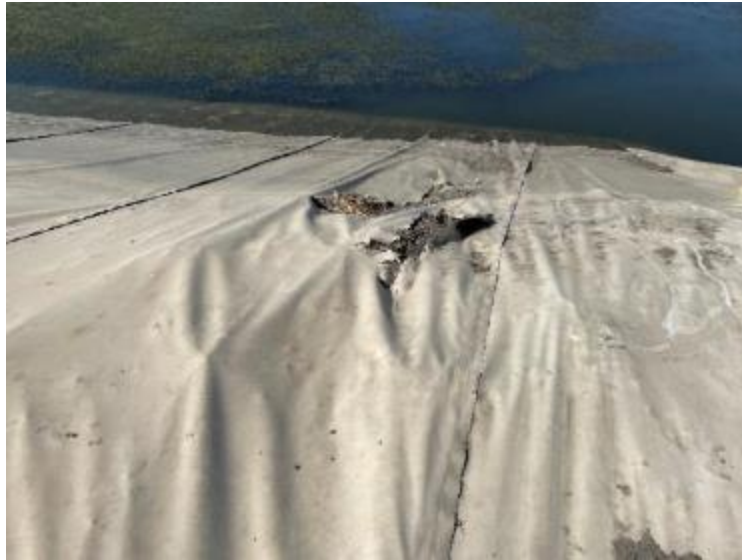
Figure 39. Puncture failure example (one of many) in existing Laguna Reservoir lining
