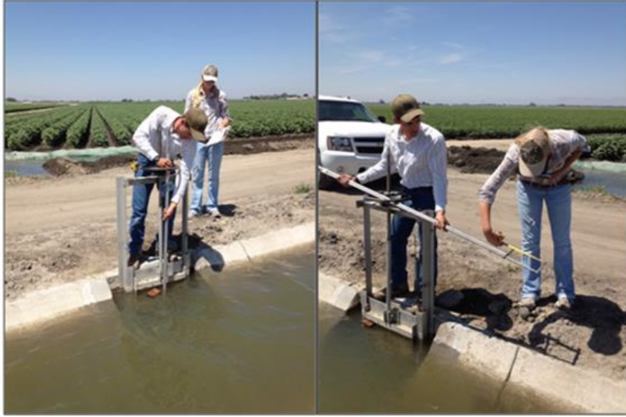
Figure 5. Special tool to detect actual gate opening
