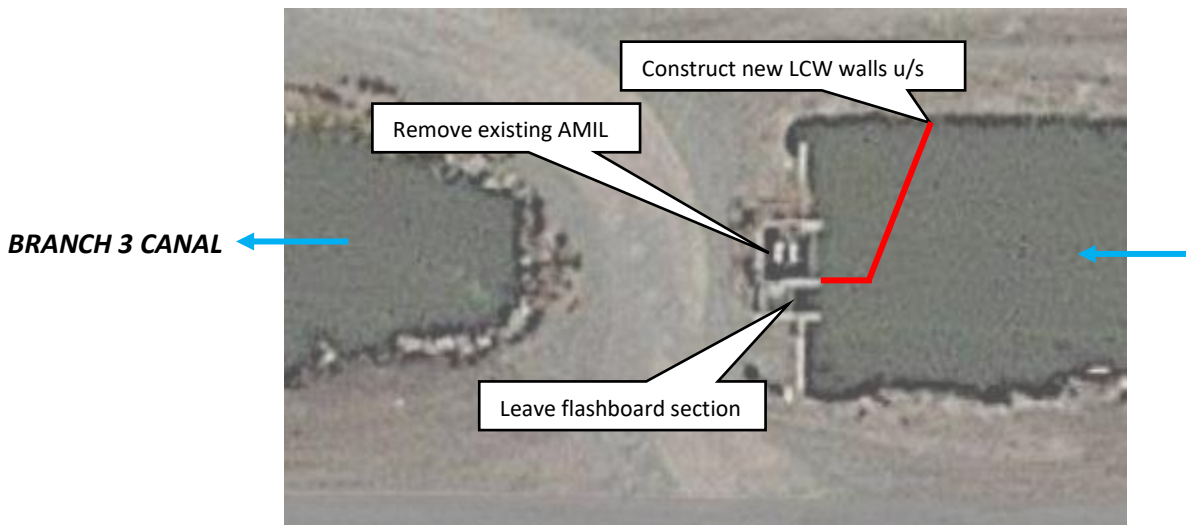
Figure 85. Conceptual LCW design to the existing AMIL gate check at Branch 3 Canal station 125+50
