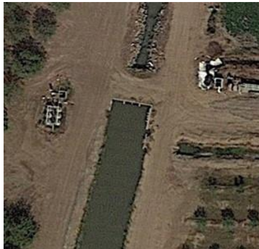
Figure 10. Satellite image of the existing, upstream flashboard structure. Note turnouts on both banks.
